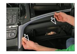
5. Unclip and remove right panel
