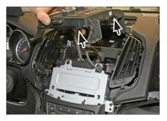
6. Remove screws of OEM head unit control unit
